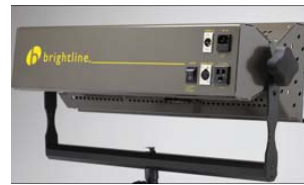
Rear of DALI Dimming Fixture showing Power In and Thru and On/Off Switch; and DALI Signal In and Thru.
