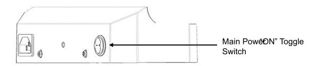
3) Press and hold down the Remote (F) ON button <u>within</u> five (5) seconds of turning ON the Main Power Toggle Switch.
