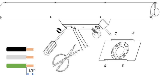
3. Connect the Black, Ground and White (L-G-N) wires from the Plug-In receptacle located in the Main Body Housing to the terminal connection box of the cMe3 as shown below.
