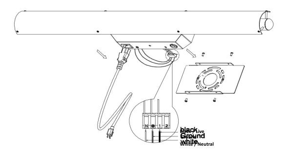
4. Remove the receptable Plug-In cover plate as shown below using a #2 Philips Screwdriver (not included).
