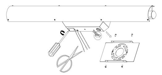
5. Install the Main Housing Canopy to the Canopy Back Plate as shown below. Be sure to tuck all wires neatly into the Main Housing Canopy and align the four slotted holes on the Main Housing Canopy with the Canopy Back Plate holes. Use Canopy Allen Wrench (E) and the four screws provided with the Main Housing Canopy to secure to the Canopy Back Plate by turning clockwise until tight.
