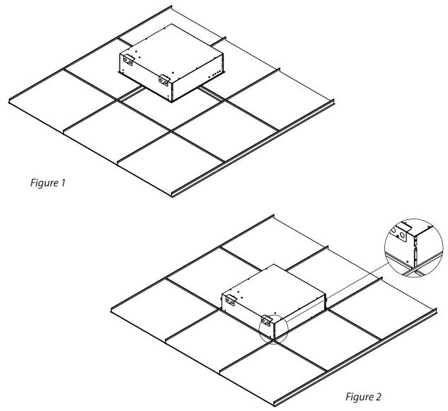
Note: Use screwdriver to bend tabs outward to install safety wires.
