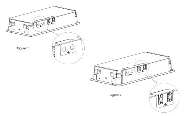
3. If the fixture requires digital control, the fixture will have locking XLR-type plugs for the control cables. Install the control wiring above the T-bar grid. Male and female plugs are installed into receptacles (Figure 2) on each fixture; as they are wired in parallel, the control wiring can be daisy-chained. See the Control Wiring section.
